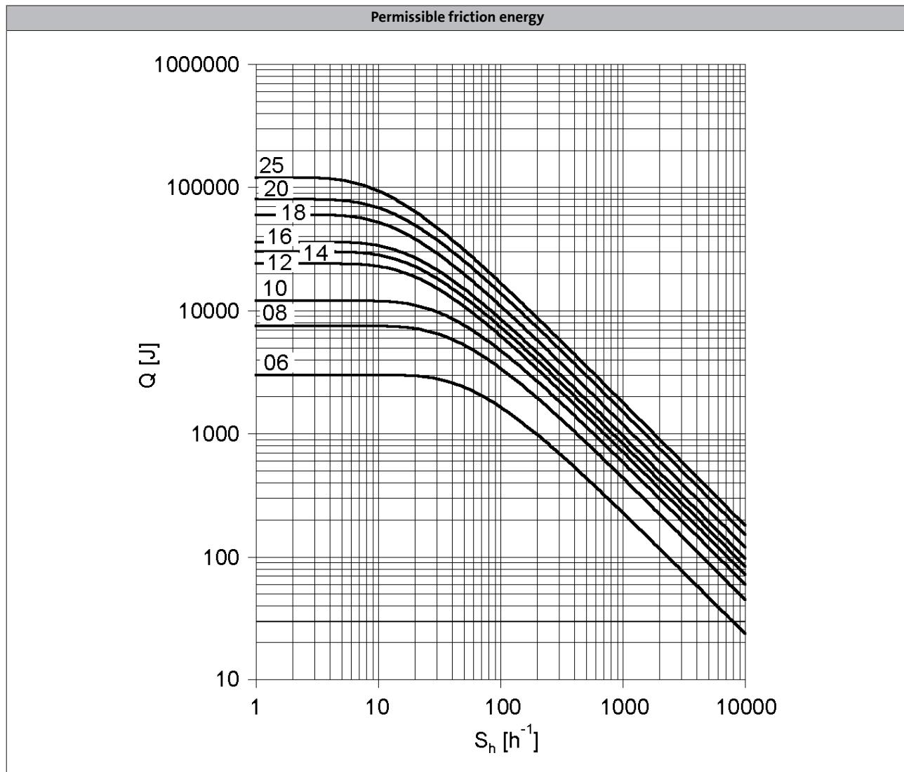
$Q$  = Switching energy per switching cycle
