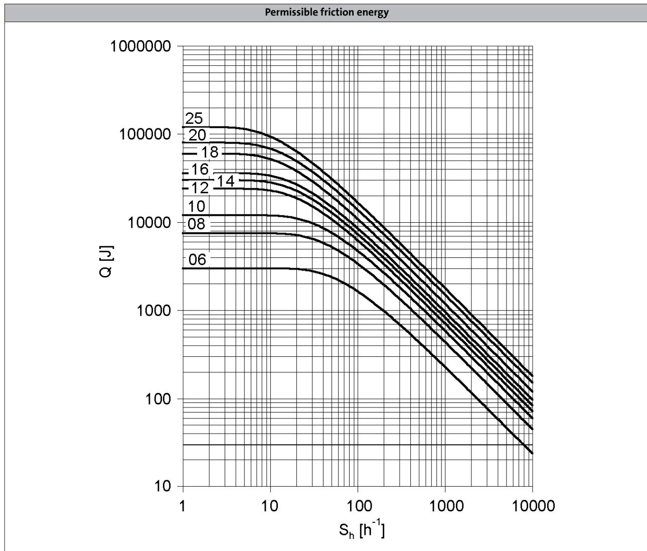
$Q$  = Switching energy per switching cycle
