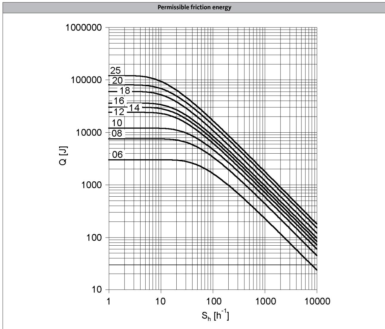
$Q$  = Switching energy per switching cycle
